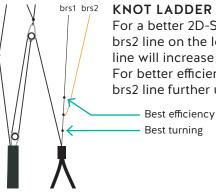
For a better 2D-Steering effect, we recommend to mount the brs2 line on the lower knot. Keep in mind that a shorter brs2 line will increase your holding and steering forces. For better efficiency and less 2D-steering effect, move the brs2 line further up the knot ladder.
